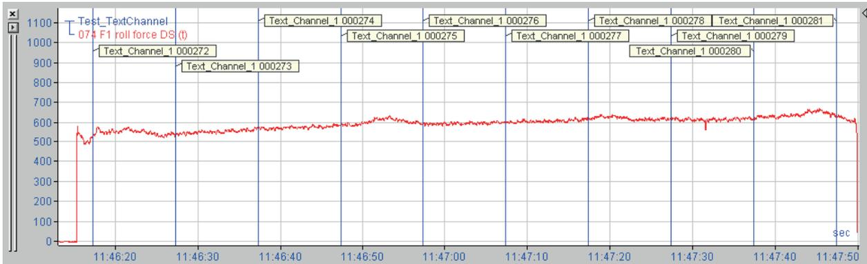
If you use *ibaQPanel* for online display on your *ibaPDA* client, the text signals can be displayed along with the *ibaQPanel* trend graph. An example for this is shown in the figure below.
