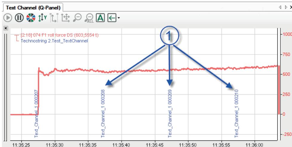
If you use an *ibaCapture* camera view either on your normal *ibaPDA* client or on an *ibaQPanel*, you can use text signals for overlay text displays. An example for this is shown in the figure below.
