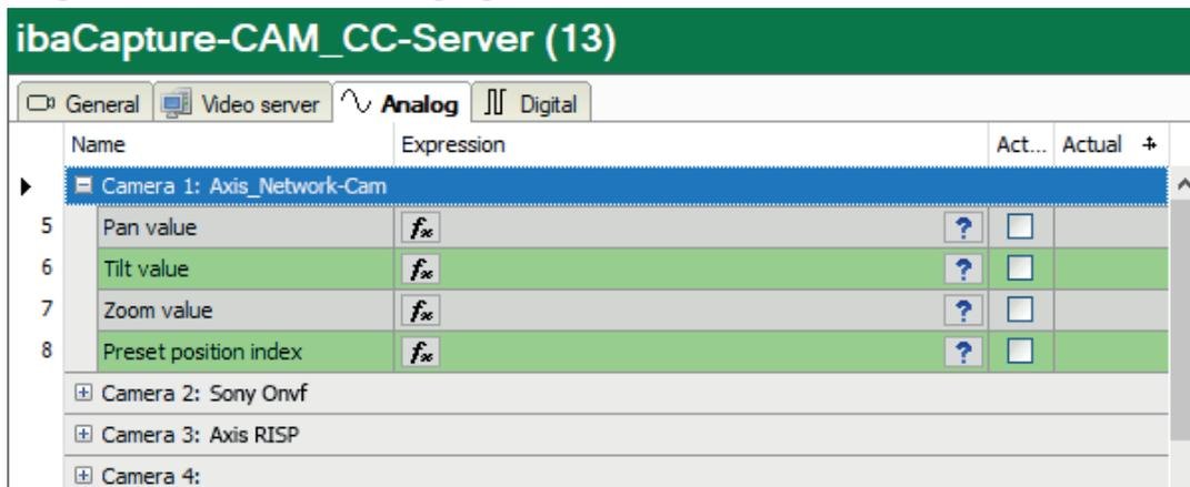
If you use PTZ (pan tilt zoom) cameras and want to control their settings in terms of pan, tilt and zoom with *ibaPDA*, you can do this by using analog output signals. You can define the values for the pan and tilt angle as well as for the zoom factor by using the expression editor. Presets stored in the camera can also be accessed directly. A data set is available for each of an *ibaCapture* server's 16 cameras.
