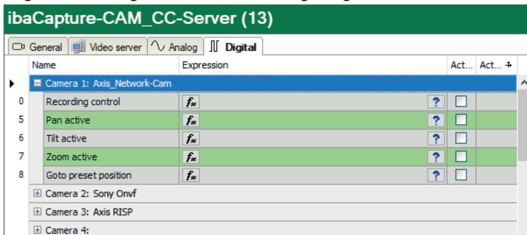
A data set with digital output signals is available for each camera of an *ibaCapture* server. You can use the first signal "Camera recording control ..." to start and stop a camera video recording. You can use the expression builder to configure the signal depending on the process. To control PTZ cameras, you will find the digital output signals to enable or disable the control functions (pan, tilt, zoom and preset) in this tab.
