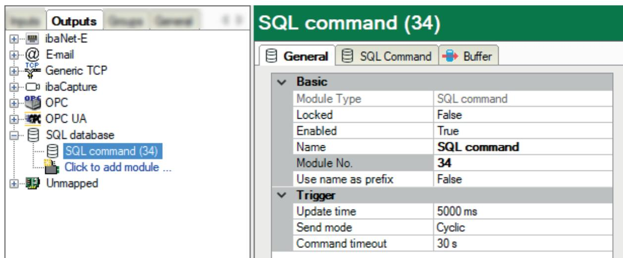
The screenshot shows the IBA configuration interface. On the left, the 'Outputs' tab is active, displaying a tree view of modules. The 'SQL command (34)' module is selected. On the right, the configuration window for 'SQL command (34)' is shown, with the 'General' tab selected. The configuration is divided into 'Basic' and 'Trigger' sections.
